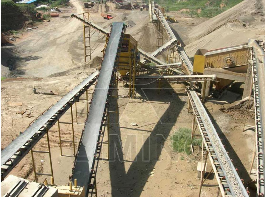
The belt conveyers produced by BREAK-DAY can be operated in the circumstance temperature range from  $-20^{\circ}\text{C}$  to  $+40^{\circ}\text{C}$ . The temperature of transferred material by this belt conveyor should be lower than  $50^{\circ}\text{C}$ .
